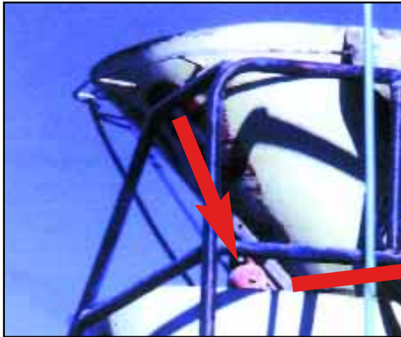
VIBCO VS-250 air vibrator mounted on the charge hopper of a front discharge mixer truck. (Complete kit available.)
